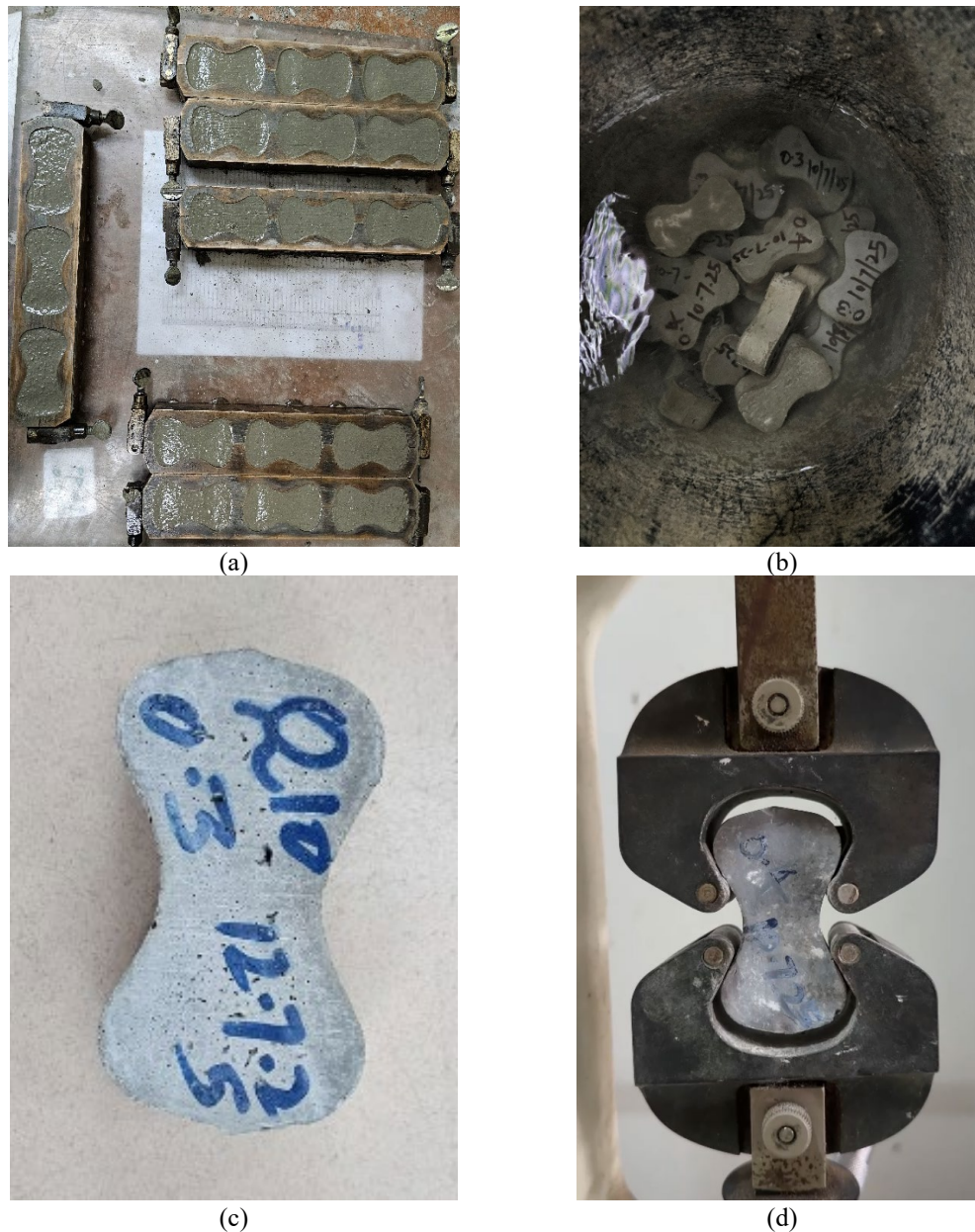
Figure 3. a) test specimens b) curing after 24 hrs, c) typical test specimens and d) test setup.
