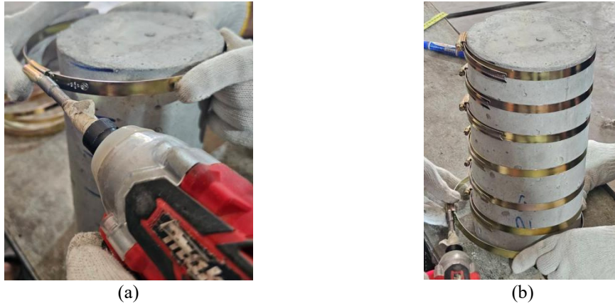
Figure 4. (a) Application of steel clamp at designated location and (b) a completely confined specimen.
