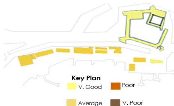
Figure 12. The buildings conditions surrounding Qaitbay Plaza, Source: AutoCAD tracing modified by
